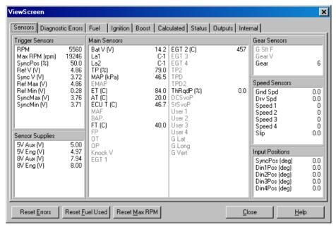
The View Screen has a number of pages that may be accessed by pressing **Tab** while holding down the **Ctrl** key or by pressing the first letter of the screen name.
