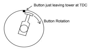
The button must be a wide tip type to cater for a wide range of advance points since the advance is changed electronically rather than mechanically.
