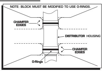
Figure 4 Modified Block for use with 0-Rings.
