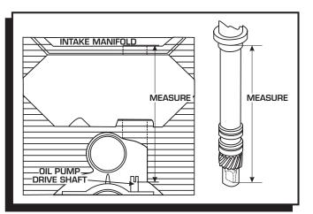
Figure 3 Measuring Oil Pump Overlap.
