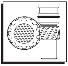
Figure 2 Correct Gear Mesh.
