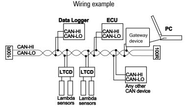
For information on wiring a CAN bus with several LTCs and any number of other CAN devices (as in the example), refer to the relevant device manual.
