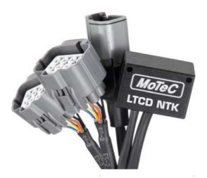
MoTeC's LTCD NTK (Lambda To CAN) is the dual version of the LTC NTK. It monitors, controls and diagnoses two NTK Lambda sensors, and transmits Lambda readings on a CAN bus. When using dual LTCs or a mix of singular and dual LTCs, up to 32 Lambda sensors can be configured on a single CAN bus to simultaneously monitor multiple Lambda sensors.
