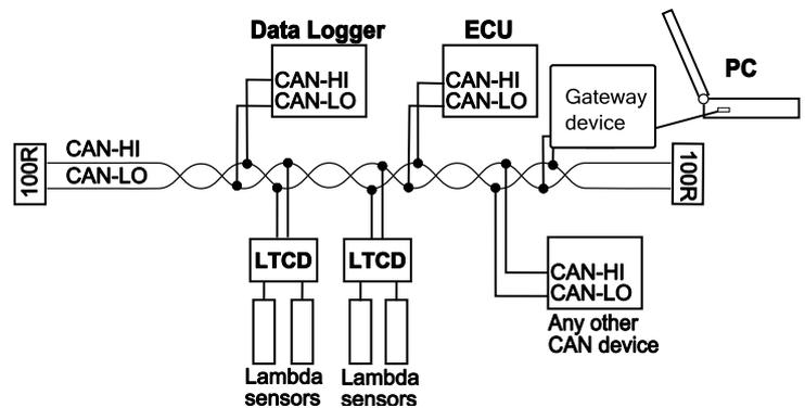
For information on wiring a CAN bus with several LTCs and any number of other CAN devices (as in the example), refer to the relevant device manual.
